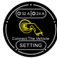
Charging standby interface
